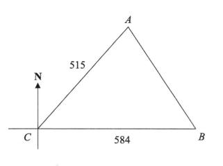
Points A, B and C are on level ground. B is due east of C. A is 515 m from C on a bearing of  $055^{\circ}$ . B is 584 m from C.
