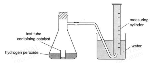
The experiment starts when the test tube is tipped so that the catalyst comes into contact with the hydrogen peroxide. The oxygen gas is then collected in the measuring cylinder.
