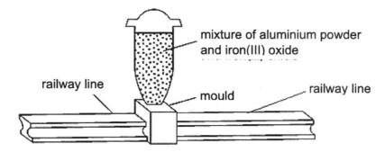
The mixture is ignited and an exothermic reaction takes place. The molten iron formed is collected in the mould. The molten iron solidifies and repairs the crack between the rails. The mould is then removed.
