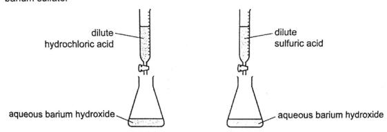
In each experiment, the acid is run into the conical flask until the pH is 7. Which are the next steps needed to obtain the solid salts?
