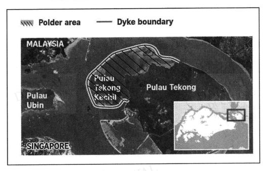
A new method of land reclamation, known as empoldering, will be used at the north-western tip of Pulau Tekong. This method involves building a dike (embankment) around the area to be reclaimed and draining water from it, creating a low-lying tract of land below sea level, called a polder. The polder is buffered from the sea by a dike, and water levels in the polder are controlled by drains and pumps.
