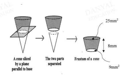
Given that the height of the frustum is 8mm and the two circular base areas of 9  $mm^2$  and 25  $mm^2$  respectively.
