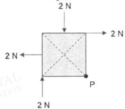
How many pairs of the forces above will give a net moment with a magnitude of S Nm?
