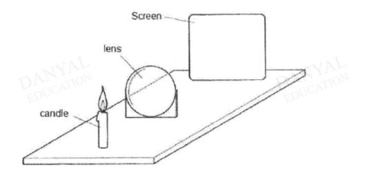
Various focussed images of the candle are produced on the screen by moving the lens and the screen backwards and forwards.
