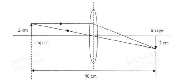
Which of the following object distance will result in a magnified and virtual image?
