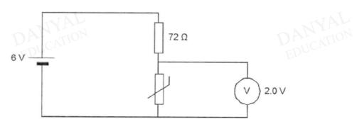
What is the resistance of the thermistor when the temperature is 20°C?
