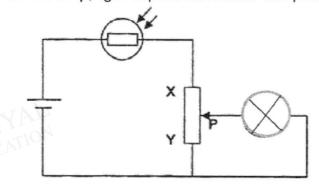
Which of the following adjustments will cause the lamp to be the brightest?
