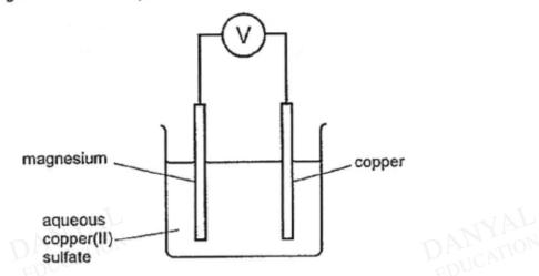
Write down the ionic half equations, including state symbols, for the reaction at the electrodes.
