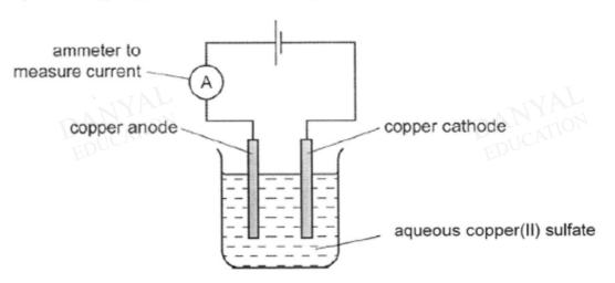
He uses the same concentration of aqueous copper(II) sulfate each time, but changes the current he passes through the solution. He runs each electrolysis for 10 minutes. The student weighs the negative electrode before and after each experiment and works out the mass of copper deposited.
