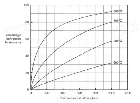
(a) A particular industrial plant uses a pressure of 400 atm and a temperature of 500°C. From the graph, determine the percentage yield of ammonia under these conditions.
