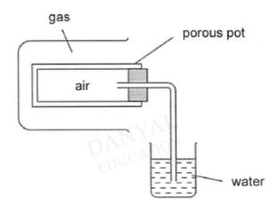
A beaker containing the gas was placed over the porous pot.
