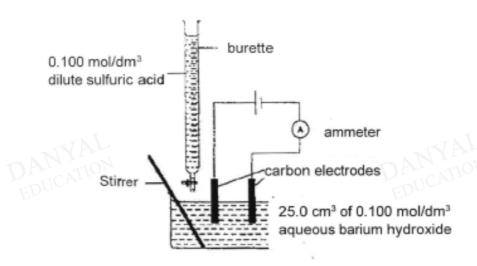
The acid was added from the burette in portions of 5 cm<sup>3</sup> until 40 cm<sup>3</sup> of the acid was added. After each addition, the solution was stirred and the ammeter reading was noted.
