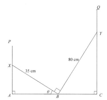
In the diagram XBY is a structure consisting of a beam XB of length 35 cm attached at B to another beam BY of length 80 cm so that angle  $XBY = 90^{\circ}$ . Small rings at X and Y enable X to move along the vertical wire AP and Y to move along the vertical wire CQ. There is another ring at B that allows B to move along the horizontal line AC. Angle  $ABX = \theta$  and  $\theta$  can vary.
